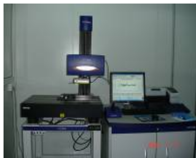
Talysurf Hobson 轮廓仪 镜片RT测试
